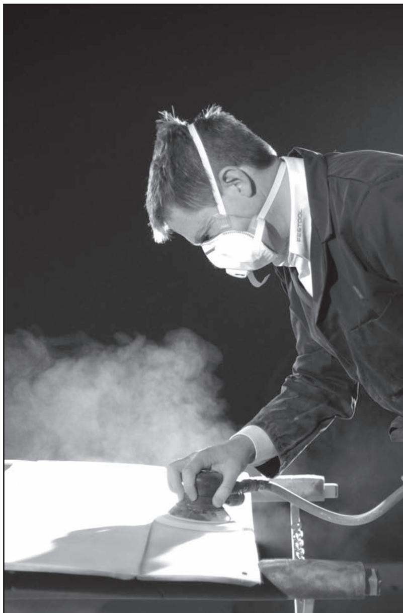
*Operative using a palm sander without on-tool extraction. Backlighting reveals the dust that is not always visible under normal conditions.*
